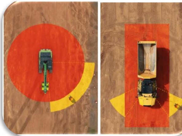
Entering from safe visibility zone
