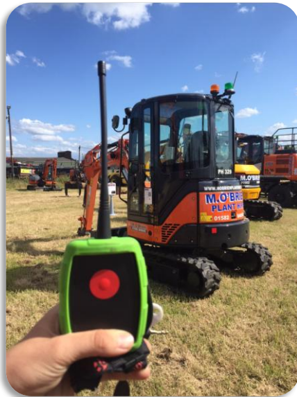
Remote cut off
